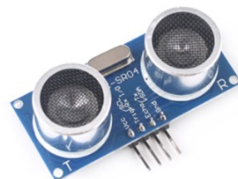
Figure 8. Ultrasonic distance measuring device.
